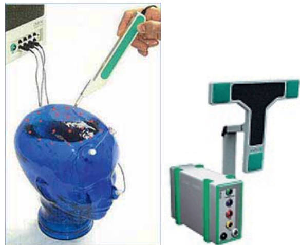
Fig. 1. Digitizer CMS20 working on the basis of ultrasonic emission
