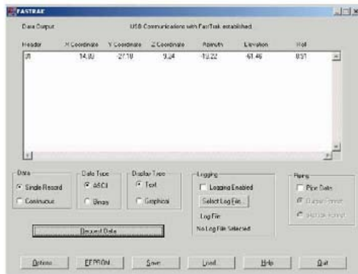
Fig. 5. Receiving data from the FASTRAK using the GUI software
